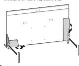
2 Remove the screws from the rear of the TV.
