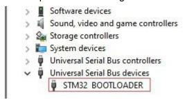
5. Before writing the firmware for the first time, you need to replace the STM32 BOOTLOADER driver to ensure that the EdgeTX Companion software can recognize this hardware type and write the firmware correctly. The replacement method is as follows:
