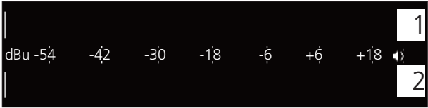
Audio level display – transmitter turned off
