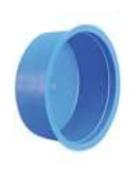
Inlet and outlet plugs are installed into the grout tubes of the coupler in order to keep dirt, water and concrete slurry out of the coupler during the concrete pour, transportation and installation.
