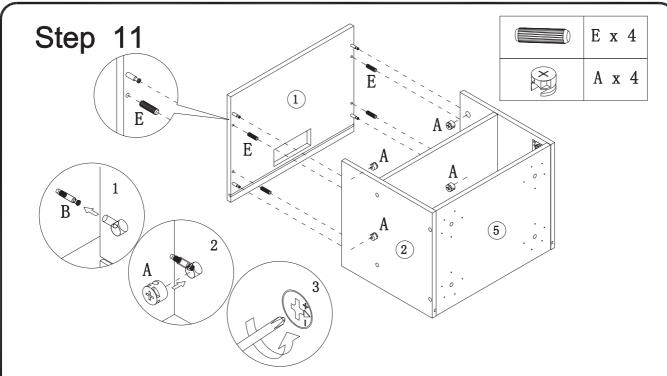
Step 11: Install E into the corresponding hole of Step 9, then attach the ① part to Step 9 with P.
