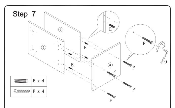
Step 7: Install E to 4 5 parts, then use F to connect 3 to 4 5 parts through O.
