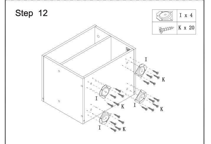
Step 12: Attach the I to the pin hole of Step 11 with K through P.
