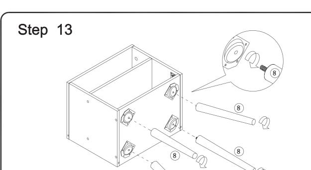
Step 13: Attach the ® part to the corresponding hole of Step 12.
