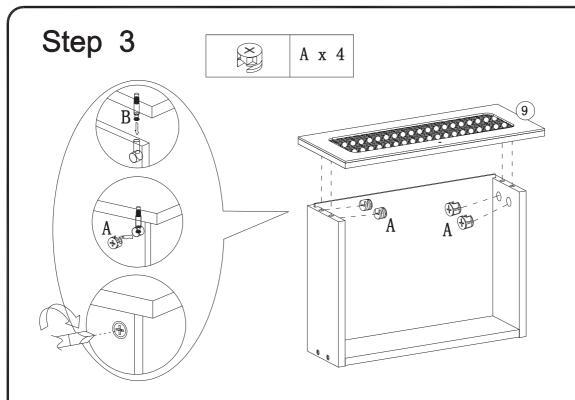
Step 3: Use P to attach the A to the Step 2 hole to connect the part ⑨.
