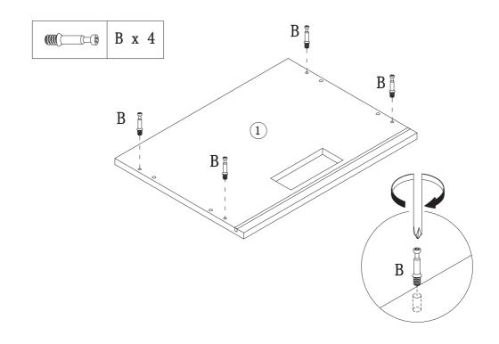
Step 10: Install B to ① part with P.
