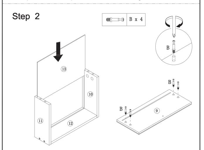
Step 2: Insert part ③ into Step 1 notch and install B to part ⑨ with P.
