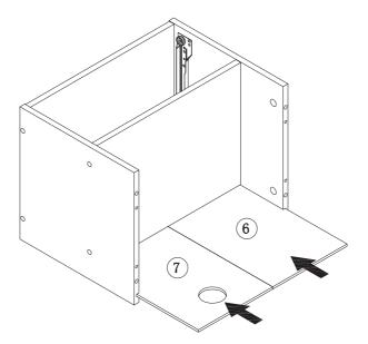
Step 9: Insert ⑥ ⑦ parts into Step 8 notch.
