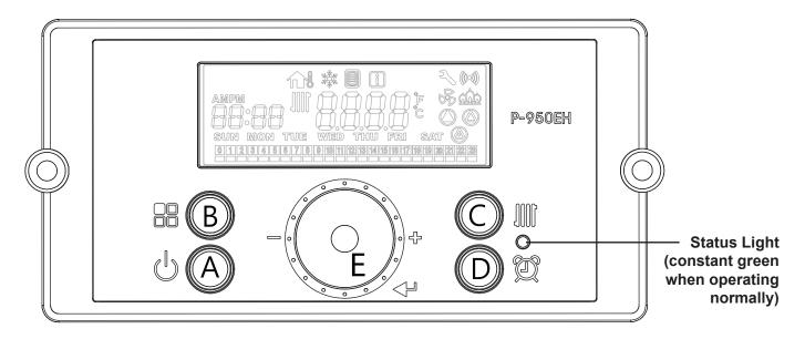
**The Control Display** has a Control Dial (E), 4 buttons (A, B, C, D), and a Liquid Crystal Display (with 72 back-lit segments). This section of this manual gives instruction on how to navigate into the many functions of the FT and to change temperature set points, set system variables and controller parameters.
