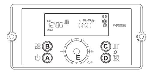
**To change CH Setpoint,** press the C button. The CH Icon and current CH Setpoint will flash.
