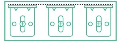
Position brackets at the right height. The longer side is to be mounted onto the wall. When drilling, we advise going through the centre of the larger middle hole, allowing for height adjustment. Predrill using the brackets as a guide.
