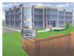
Geothermal closed loop
