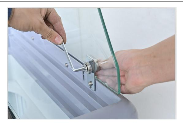
NOTE: The small and large screws are not suggested to fasten tight firstly, so you can install the front glass panel easily by adjusting the position of the two side glass panels. White plastic washers will be put in the middle of Large screws.
