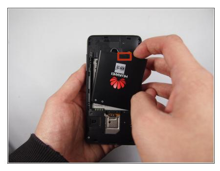
• Lift up and remove the battery for replacement.
