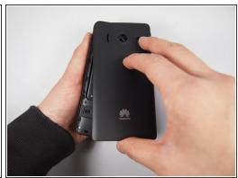
• Remove the rear cover at the back by pulling the gap located at the bottom of the phone.
