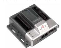
The VEX ARM® Cortex®-based Microcontroller coordinates the flow of information and power on the robot. All other electronic system components must interface to the Microcontroller - it is the "brain" of a robot
