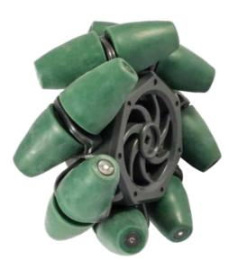
Mecanum Wheels allow savvy robot designers to create drivetrains capable of moving in any direction using a standard chassis shape. Simply power each wheel with its own independent motor by changing the directions the wheels spin, your robot can now move sideways!
