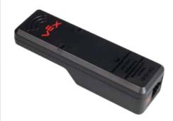
The beauty of a reliable radio connection, in a small simple package. The V5 Robot Radio allows your V5 Robot Brain to communicate with other devices. All wireless communication to the V5 Robot Brain is done through the V5 Robot Radio, including competition control and wireless activation of VEX Coding Studio programs.
