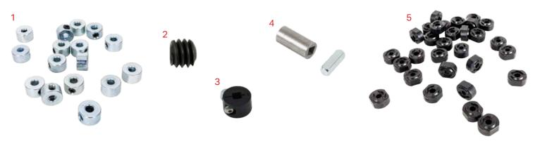
Collars lock to drive shafts, keeping wheels and gears from sliding along the shaft. Standard Shaft Collars are fastened in place using a set screw, while Clamping Shaft Collars use standard VEX EDR button head screws and nuts to maintain a tight lock without scratching or damaging the shaft. Rubber Shaft Collars easily slide onto VEX EDR 0.125" shafts and use friction between to keep wheels and gears in place.
