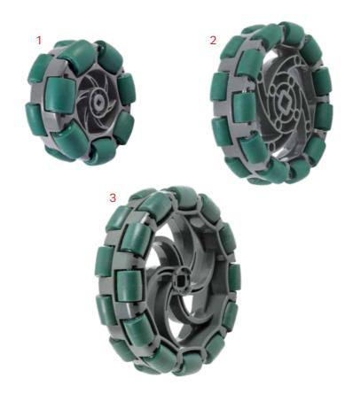
Defense may not always win championships, but being able to move does. Put some power on the floor with our large variety of wheel options available for builders. Omni-Directional wheels roll forward like normal wheels, but slide sideways with almost no friction (no skidding during turns). Use these wheels to make your robot turn smoothly or build a holonomic drivetrain.
