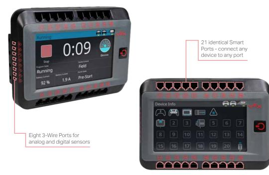
Everything centers on the V5 Robot Brain. The color touchscreen makes the V5 Brain familiar and easy to use without needing a manual. Connect your motors and sensors to any of the 21 smart ports. You can even use existing Cortex sensors by connecting them to the additional eight 3-Wire ports. A graphical dashboard is built-in for every connected device, providing incredible teaching and diagnostic capability.
