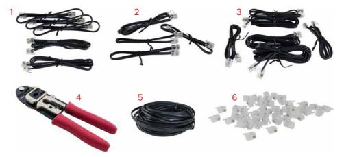
V5 Smart Cables allow robot components such as motors and sensors to communicate with the Robot  $Brain. \ These \ are \ available \ to \ purchase \ at \ pre-cut \ short \ and \ long \ assortments, or \ create \ your \ own \ custom$ length wires with the V5 Crimping Tool!
