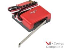
These switches are great for detecting subtle events, such as when a robot arm has reached the top or bottom of its motion.
