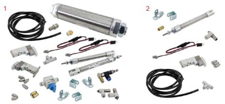
Pneumatic cylinders use compressed air (rather than motors) to produce motion that rests in one of 2 states: fully extended or fully retracted. Pneumatics Kits 1 and 2 are complete pneumatics systems for use on VEX EDR robots; Kit 1A and 2A add-ons cannot be used without a Kit 1 or 2.
