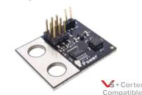
Measures accelerations on three axes simultaneously. By measuring the acceleration of the robot, one can calculate the velocity of the robot or the distance this robot has traveled.
