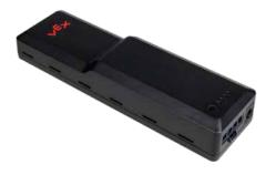
This lithium-ion battery has enough power to run ten V5 motors at full power continuously. Built-in electronics handles charging, cell balancing and precise capacity measurement. Check your battery level with the press of a button. Charge time is approximately 60 minutes, and you can even use the Brain while the battery charges.
