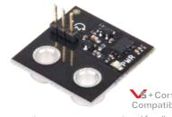
Enhances autonomous movement and feedback from a VEX robot by detecting a robot's rotation from its origin on a single axis.
