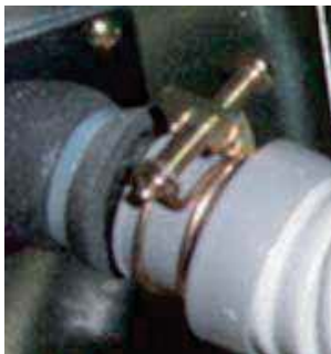
Clamp the Flexible Drain Hose Connection
