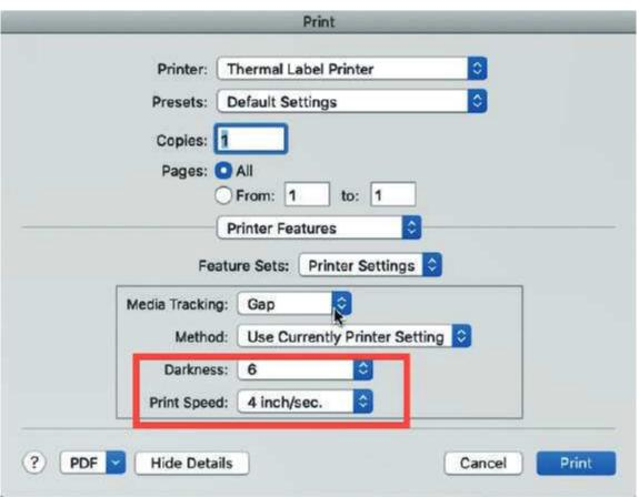
Tips: The darkness, larger number means higher darkness. If labels print out light, you can adjust it to large value, 2-4 is recommended.
