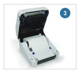
Put the roll label in or insert the fan-fold label from outside at the tear-off point, adjust the paper guide to fit the width of paper
