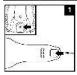
Insert the charging adapter plug into the port on the handle.
