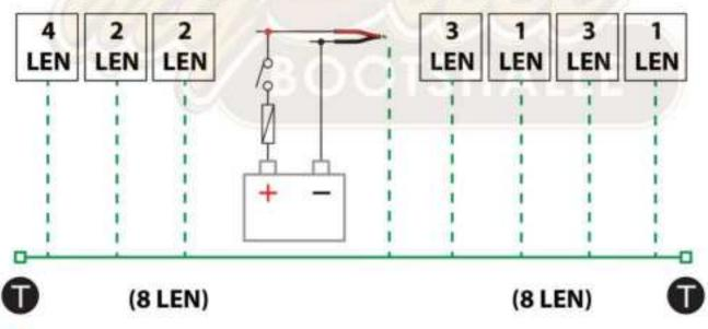
Note: Do not connect the NMEA 2000<sup>®</sup> power cable to the same terminals as the engine start batteries, autopilat computer, bow thruster or other high-current devices.
