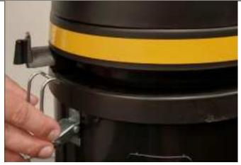
Ensure that the drain hose bung is correctly fitted and sealed. (9000 only)
