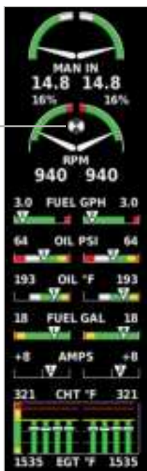
Example Engine Indication System (Multi-Engine)
