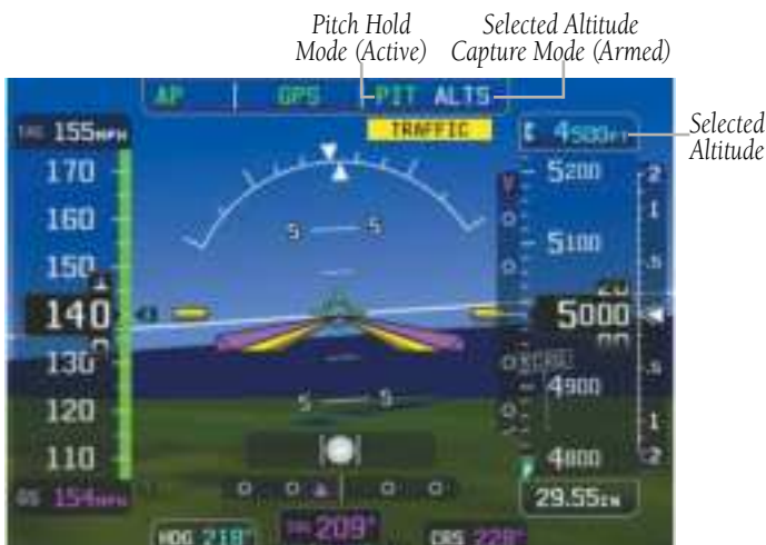
Pitch Hold & Selected Altitude Capture Modes
