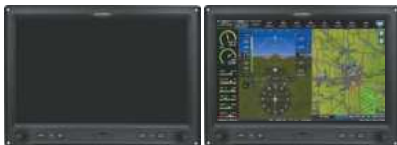
G3X Touch Full-Screen Reversionary Mode (Failed PFD)
