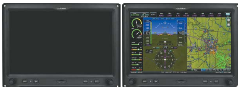
G3X Touch Full-Screen Reversionary Mode (Failed PFD)
