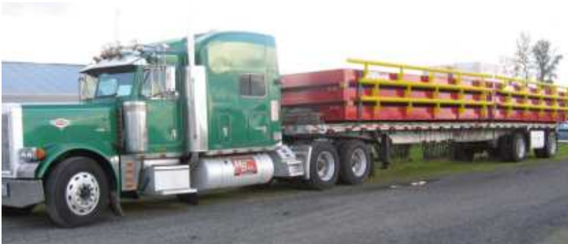
Figure 3-2. Weigh Modules Ready for Removal and Installation
