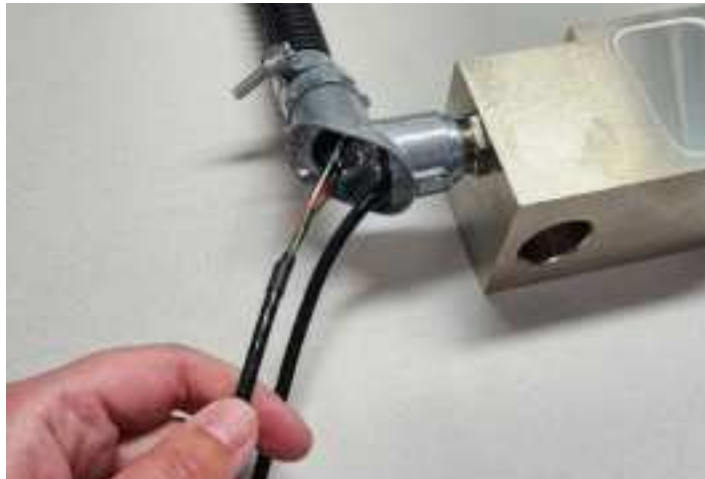
Figure 4-4. Installing 90° Fitting to Load Cell
