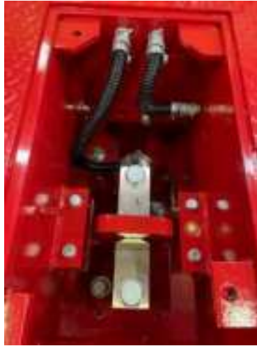
Figure 4-5. Load cell Access
