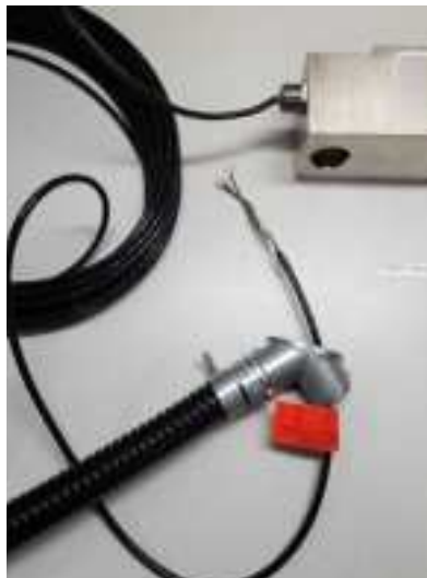
Figure 4-2. Insert Load Cell Cable Through 90° Fitting
