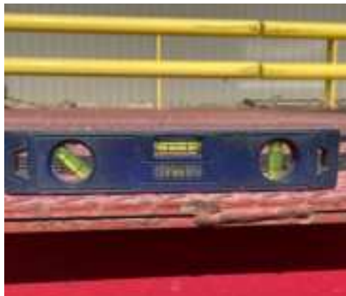
Figure 3-8. Check Weighbridge for Level
