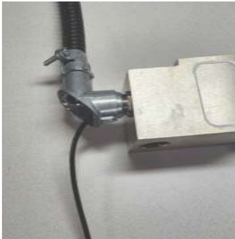
Figure 4-3. Installing 90° Fitting to Load Cell
