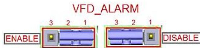
**The VFD Alarm will trigger when the contacts are open and the VFD Alarm is enabled.**
