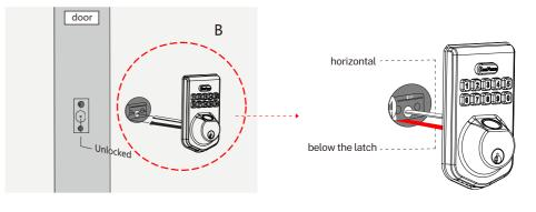
B Install mounting plate with two screws (G) provided.
