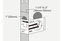
Measure to confirm the backset is 2-3/8" or 2-3/4" (60mm or 70mm). And adjust the length of the latch accordingly.
