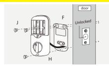
Load 4 batteries and install the battery cover.
