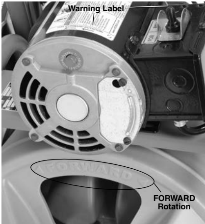
Figure 8 – Proper Drum Rotation (FOR Switch Position)
