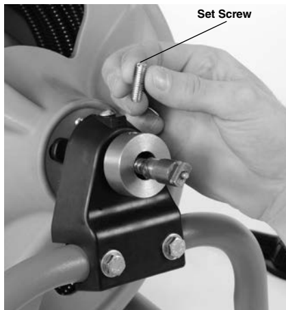
Figure 3 – Remove and discard the Cable Lock Set Screw
