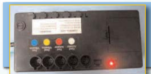
Figure 4: A flashing red LED indicates the control box has received the remote control frequency
