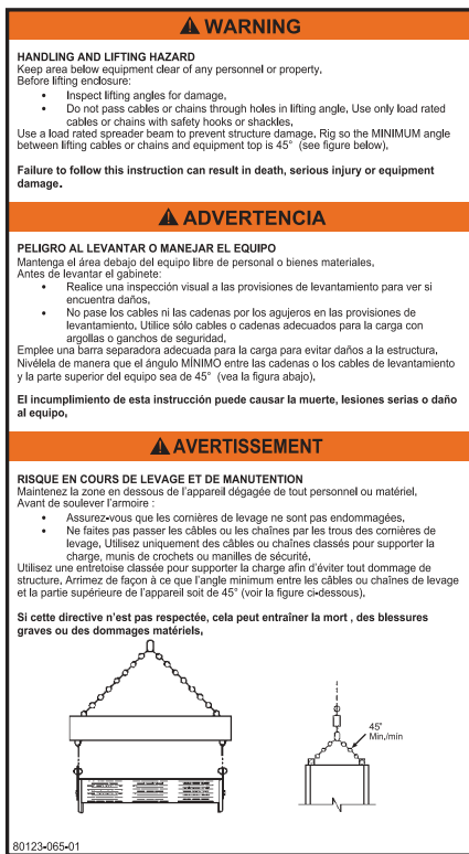
Label Applied Adjacent to Lifting Angles
