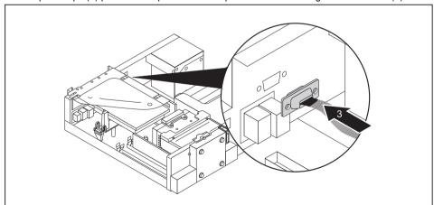
▶ Position the serial port on the inside of the device at the appropriate place (3).
