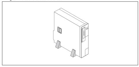
▶ Stand the device on the feet as shown.
