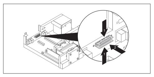
▶ Keep the clips (1) pressed and push the metal plate out of the casing from the inside (2).
