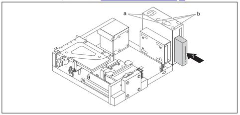
▶ When installing 2.5" HDDs/SSDs or a SmartCard reader: Connect the cables to the drive before you slide it into the bay.
