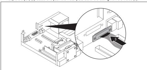
▶ Position the parallel port on the inside of the device at the appropriate place (3).
