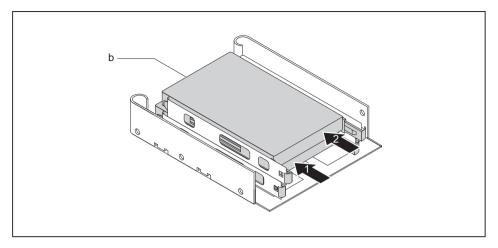
► Slide the drives with the EasyChange rails one after the other into the adapter (1, 2). In doing so, make sure that the component side of the drives point down towards the adapter and the ports on the drives are located at the rear as shown (b).
