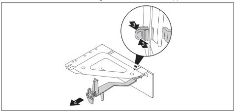
▶ Press together both ends of the display adapter support (3) and release the display adapter support from the riser card (4).
