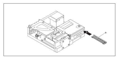
▶ Slide the drive plate (a) into the upper bay (5) again as shown, until it engages.
