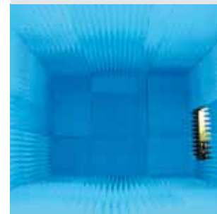
Pyramidal foam inside an anechoic chamber to eliminate internal signal reflections when testing Broadband Radar
