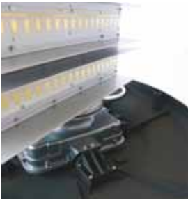
The dual microwave stripline arrays inside of the antenna dome allow continuous transmission and reception, unlike conventional radar that only has one antenna used for both.
