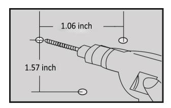
II.Insert the three plastic wall anchors to the three holes.
