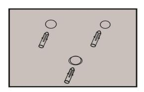
III. Fixed the bracket by three ST4\*35 screws and make sure the installation points fixed securely.
