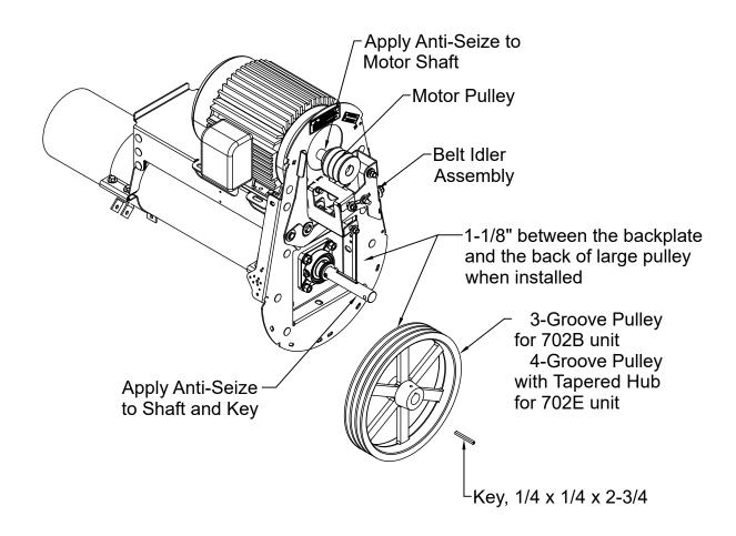
Apply Anti-Seize compound to the Motor Shaft. Install the Motor Pulley (ordered Separately), onto the Motor Shaft. Align with the large Pulley and tighten in place. Re-install the Outer Bearing Mount (removed earlier) onto the end of the Flipper Shaft and fasten it securely to the bracket on the Backplate Assembly. Tighten the setscrews of the bearing to the Flipper Shaft.
