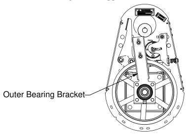
Check the Belt Guard, There should be (2) 1/4" x 5/8" Bolts in the flange of the Belt Guard that interlock with the Backplate. If they are not there, it is recommended that some be installed. These help the Latch hold the Belt Guard in place when latched.
