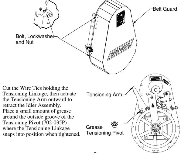
Install the Drive Belts D-3863 (BX62 Cogged Belts for 702B-001A) or D-3887 (BX64 Cogged Belts for 702E-001A). Note Clockwise Rotation.
