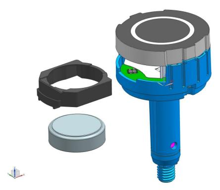
The Wireless Locker Lock includes a provision for a sliding contact via the battery replacement compartment. This contact provide access to the controllers communication and programming port. Via this port, diagnostics can be performed, configuration can be done and firmware updates can be executed.
