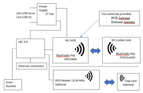
A person enters the number of the relevant Locker at the terminal and the door is opened, when touching the W1 locker lock.
