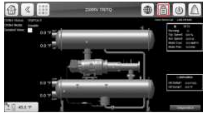
Fig. 39 — 23XRV TR/TQ Home Screen Lock Icon
