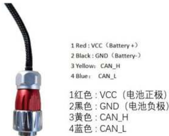
Figure 3.1 Schematic diagram of aviation plug
