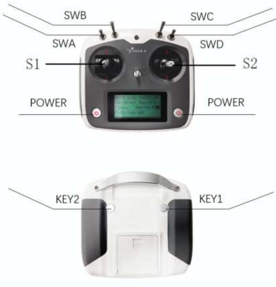
Figure 2.3 Schematic diagram of FS remote control buttons
