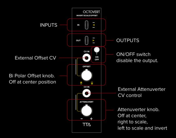
In the following patch example, Octovert is used to invert the Octostages envelope before sending it to the Octopass filter. Since the Octostages CV input operates at 0–5V, which is the standard for all Polyphonic modules, we need to adjust Octovert accordingly.
