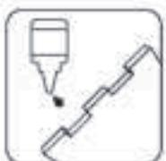
Most joints are press-fit, but some joints might require a drop of glue to ensure a strong bond.
