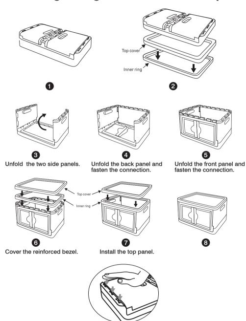
Before the assemblement, please check the each connection is correct or not; If the connection is loose, please press the folding storage box to ensure that it's more solid (You can also refer the picture)
