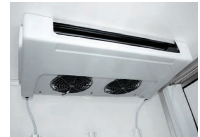
Evaporator, freezer truck
