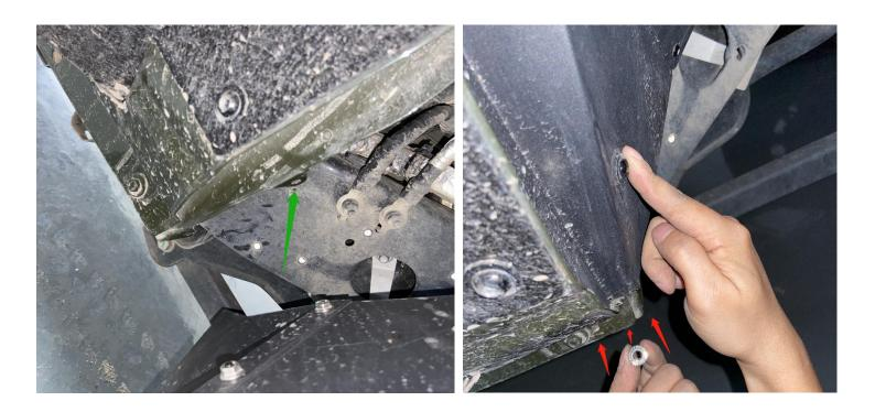
Step 12: Tighten up those bolts together. Repeat the same installation in the driver side.
