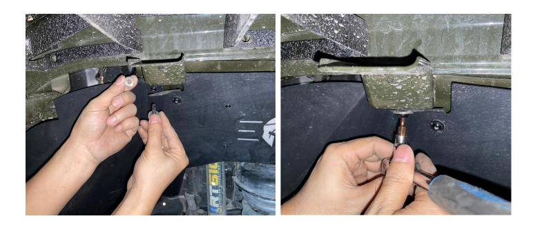
Step 10: To install the right hole. Push it inside before you screw bolt. Align the hole and screw the bolt. Use the button head socket cap bolts screws (M6\*25), flat washer (M6\*16\*1.5). Don't tighten up bolt.
