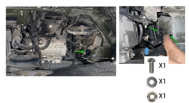
Step 9:Firstly, to install the upper two holes. you need a helper to lift up it when you screw those bolts. Use the button head socket cap bolts screws (M6\*25), flat washer (M6\*16\*1.5), Flange Hex Lock Nuts (M6). Don't tighten up those bolts.
