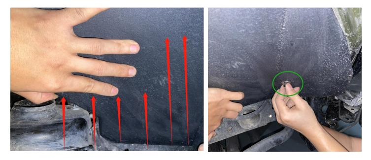
Step 11:To install the left hole. The nut needs to be inserted from underneath. Use the button head socket cap bolts screws (M6\*25), flat washer (M6\*16\*1.5), Flange Hex Lock Nuts (M6).
