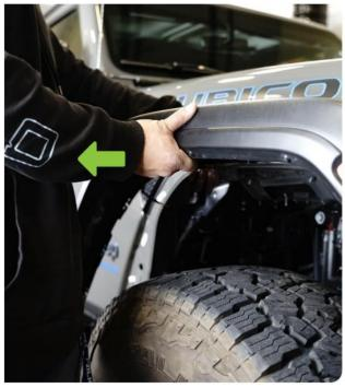
Step 4: Use a trim clip tool to remove the factory clips along the fender. Repeat process for the other side.
