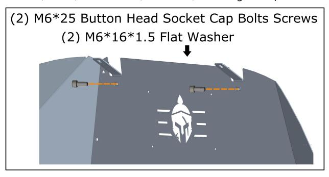
Step 8: To install the mounting bracket (2). Use the button head socket cap bolts screws (M6\*16), flat washer (M6\*16\*1.5), Flange Hex Lock Nuts (M6). The nut needs to be inserted from underneath. Don't tighten up those bolts.
