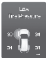
Low Tire Pressure / Tire Pressure Monitor / TPMS Malfunction Display (shown on the cluster LCD display)
