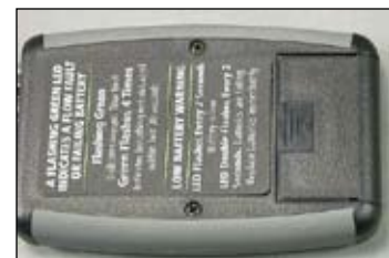
Figure 27 - OPC Back Battery Cover Installed
