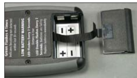
Figure 29 OPC Batteries Removed
