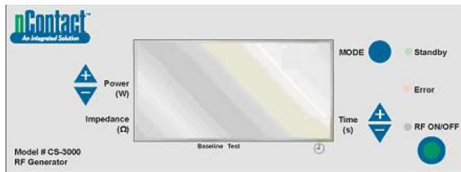
Figure 8. RF Generator Front Panel Display at “Power On”
