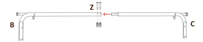
(2). Connect #A (Leg) to #B (Left Top Bar) and #C (Right Top Bar) respectively by using four sets of #T (M8\*110mm Bolt Set).
