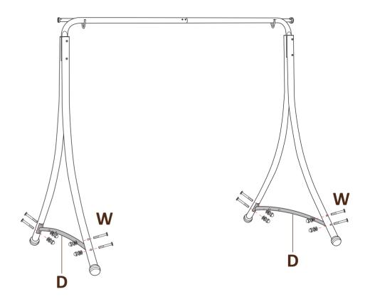
(4). Connect **#L** (Left Bottom Support) and **#L1** (Right Bottom Support) with two sets of **#Z1** (M6\*30mm Bolt Set)
