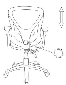
To adjust the back height of the chair turn knob counterclockwise to loosen and adjust back height. Once at the desired position, turn knob clockwise to tighten and secure back into place.
