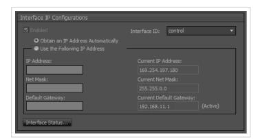
IP address, net mask (subnet range), gateway, and DNS settings may be assigned to each interface as a static setting or be provided to each interface by DHCP.
