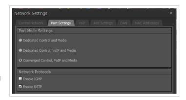
It is always safe to connect to P1 for Tesira device discovery, as long the PC and the device are in a common IP address range.
