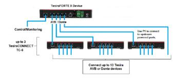
NOTE: To avoid malfunctions and potential damage to this product, it is important to understand the correct way to connect the network ports of a TesiraCONNECT TC-5, TesiraCONNECT TC-5D, and TesiraFORTÉ X to other network devices. Please read and follow these instructions carefully before connecting these products to a network:
