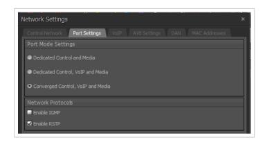
negotiated and applied. RSTP must be enabled on all network devices to work properly.
