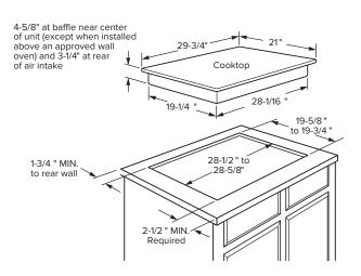
To ensure accuracy, it is best to make a template when cutting the opening in the counter
