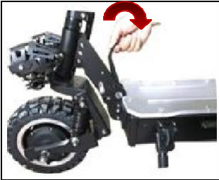
Step 1 Pull down the safety Lock
