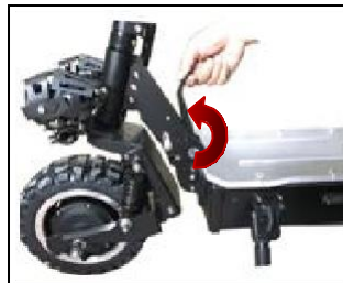
Step 2 Push back the Safety Lock
