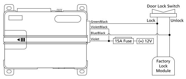
Type B: (-) ground controlling factory relays/modules
