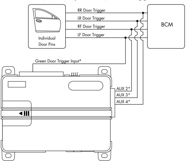
\* Default is N/O and must be programmed for N/C when connecting to Normally Closed door trigger circuits.
