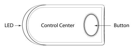
The Control Center, typically located on the upper part of the front windshield. It consists of:
