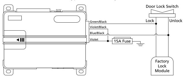
Type C: Direct wired reversing polarity
