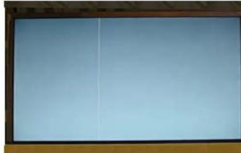
Vertical Line Source TAB IC Defect
