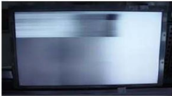
Horizontal Block Gate TAB IC Defect
