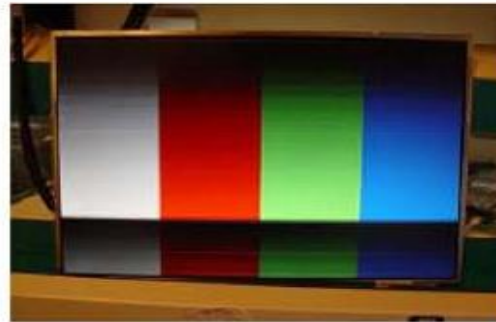
Horizontal Block Gate TAB IC Defect
