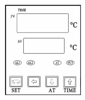
The top display, PV displays the cabinet temperature.
