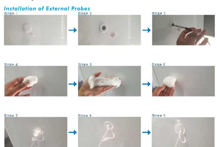
Never install probes through the door as this will prevent the door from closing properly, thus preventing a correct seal from forming and from preventing the cabinet from maintaining the correct temperature. This will damage the door gasket which will prevent a correct seal from forming.
