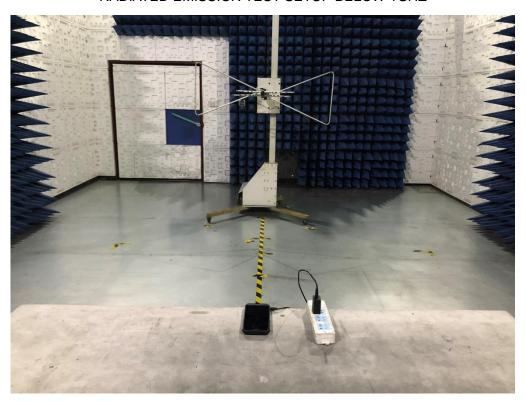
RADIATED EMISSION TEST SETUP ABOVE 1GHZ
