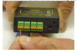
best, but if you use stranded wire be sure to twist the strands tightly together. Push the wire into the desired barrier block connection as shown. There is a common, normally open and normally closed connection for each output.
