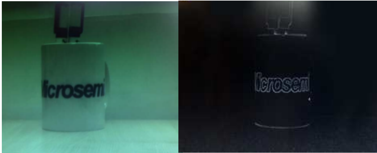
Figure 19 • Normal Image vs. Edge-Detected Image—Example 2
