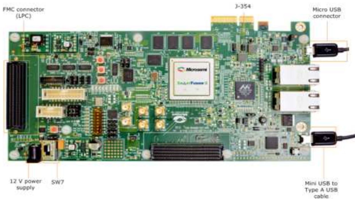
Figure 8 • SmartFusion2 Advanced Development Kit Setup
